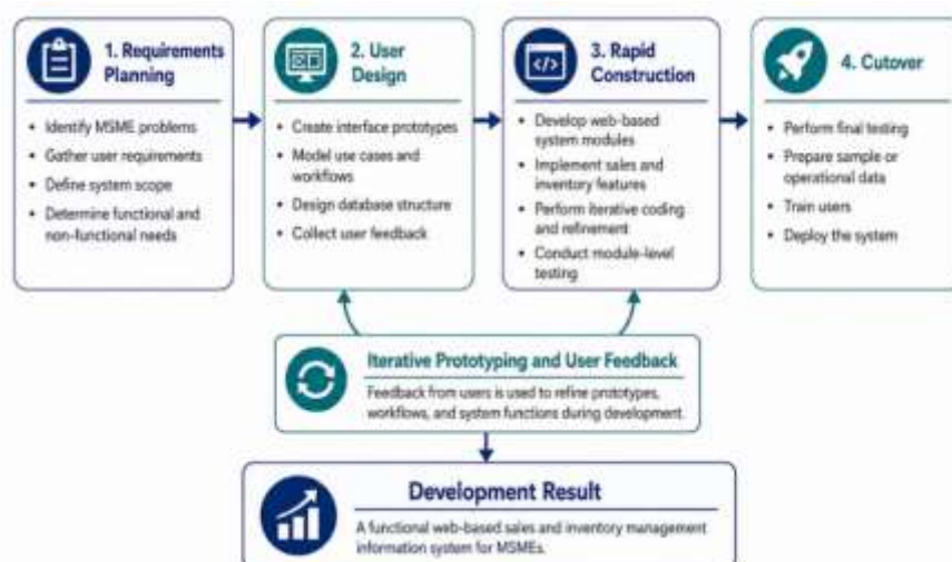
Figure 2. Rapid Application Development stages used in the development of the web-based sales and inventory management system
